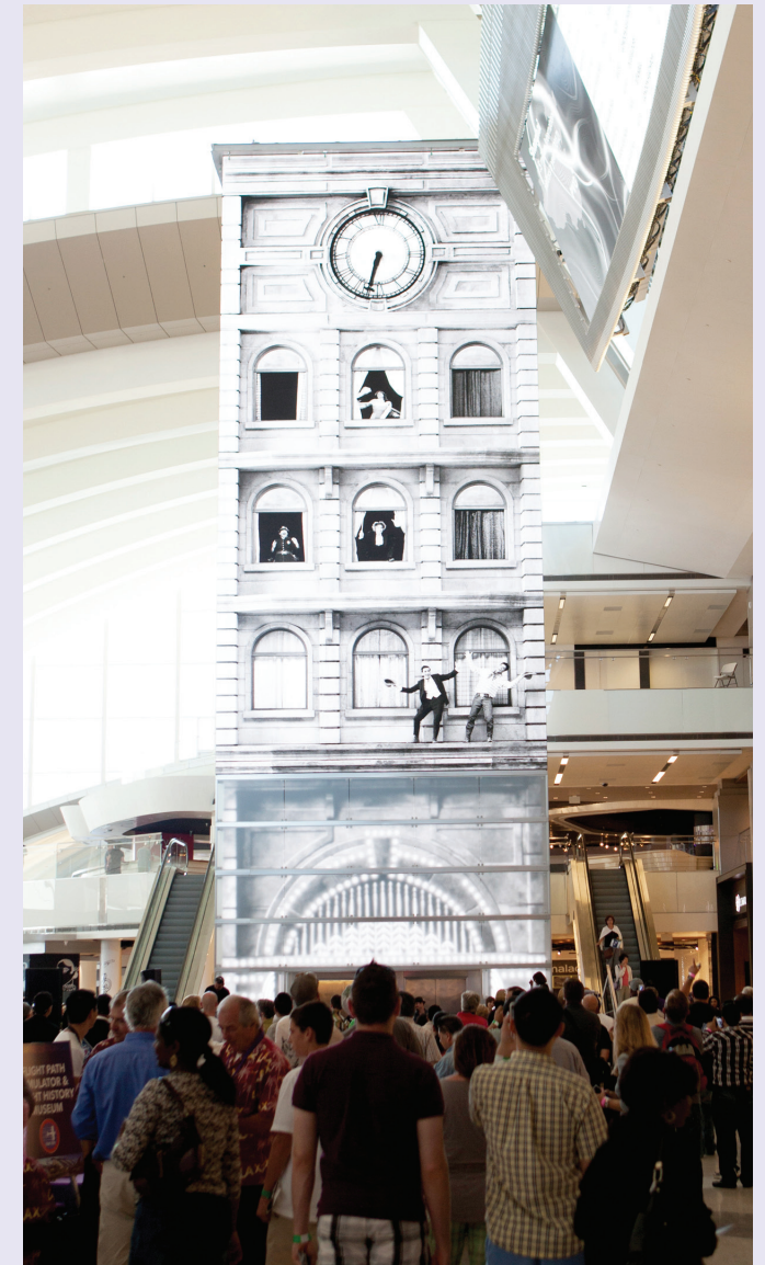
✈️ The Time Tower was conceived as a four-sided mediascape wrapped around an existing elevator core. Here it displays a short film inspired by comedy actor/producer Harold Lloyd. Moment Factory built a full-scale model and shot live-action film for the short. A functional clock face is also integrated into the tower. (Photo: Moment Factory)
