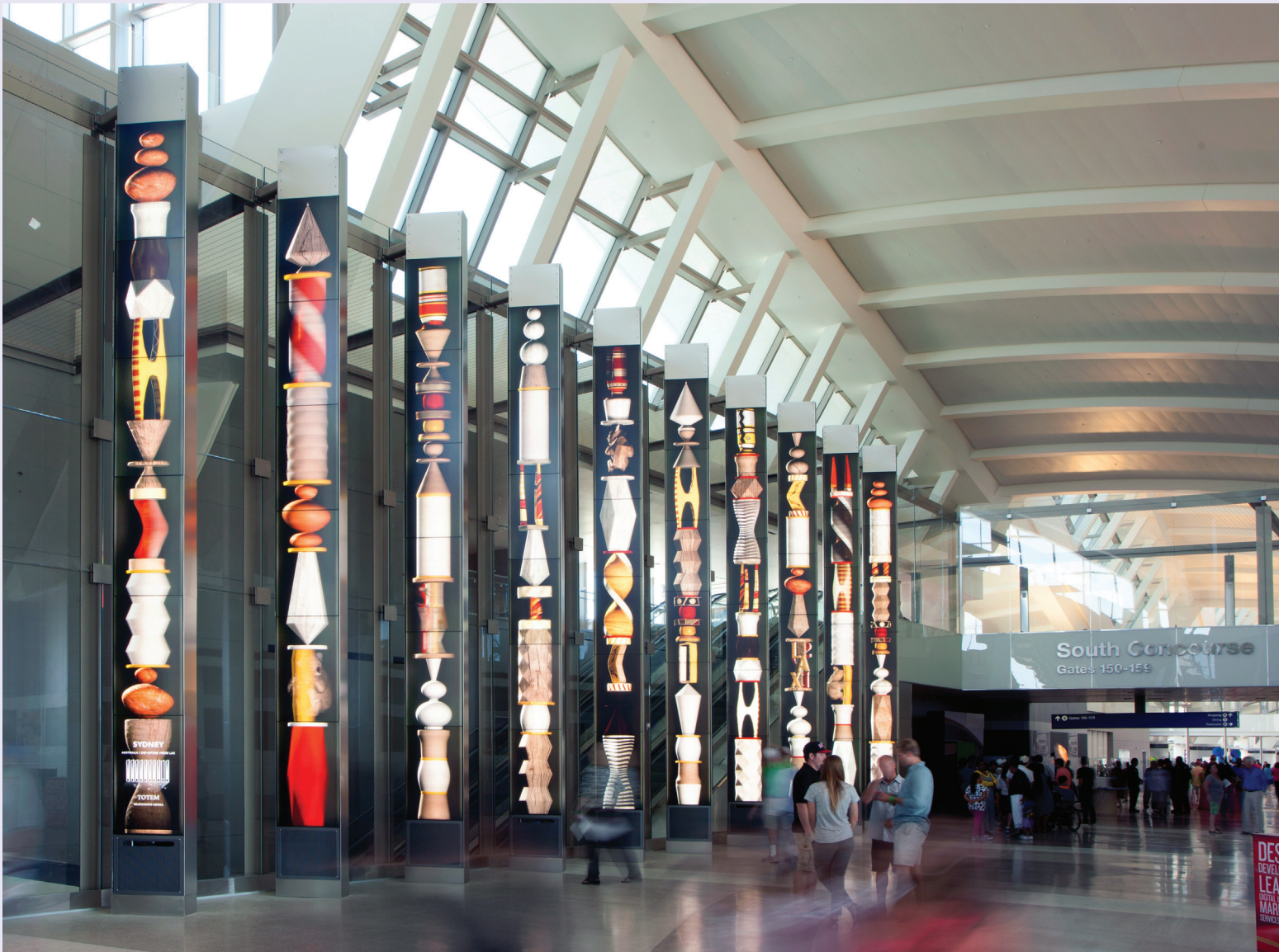
✈️ A series of 28-ft.-tall pylons provide a transitional experience as passengers move toward the North or South concourses and their departure gates. The slender monoliths consist of vertically stacked LCD monitors with content keyed to the art traditions of destination cities. Passenger movement triggers changing visual effects. (Photo: Moment Factory)
